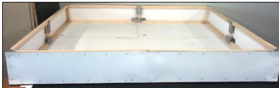
Figure 4.2: Walls Added to the Scale Model Building
