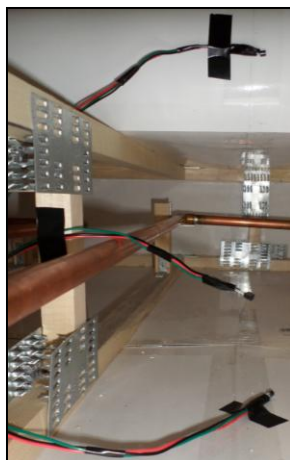
Figure 4.22: Internal Placement of Thermistors Inside the Modeling Building
