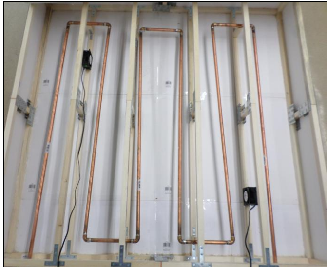
Figure 4.19: The Inside Components of the A/C System
