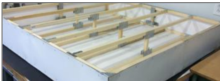
Figure 4.3: Support Beams Added to the Frame of the Scale Model Building
